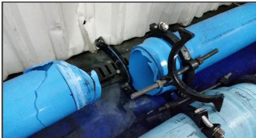
Figure 1. Brittle failure of spigot at 400psi
