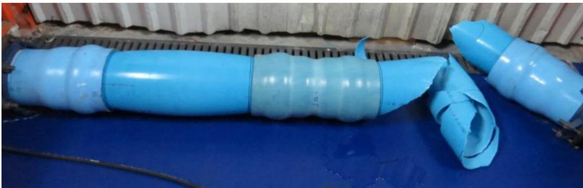
Figure 4. Pipe burst away from the joint.
