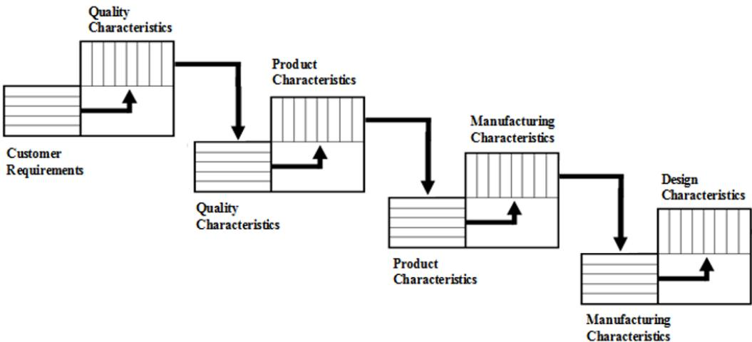
Figure 1: The Structure and Flow cascade of Quality Function Deployment (aka House of Quality)
