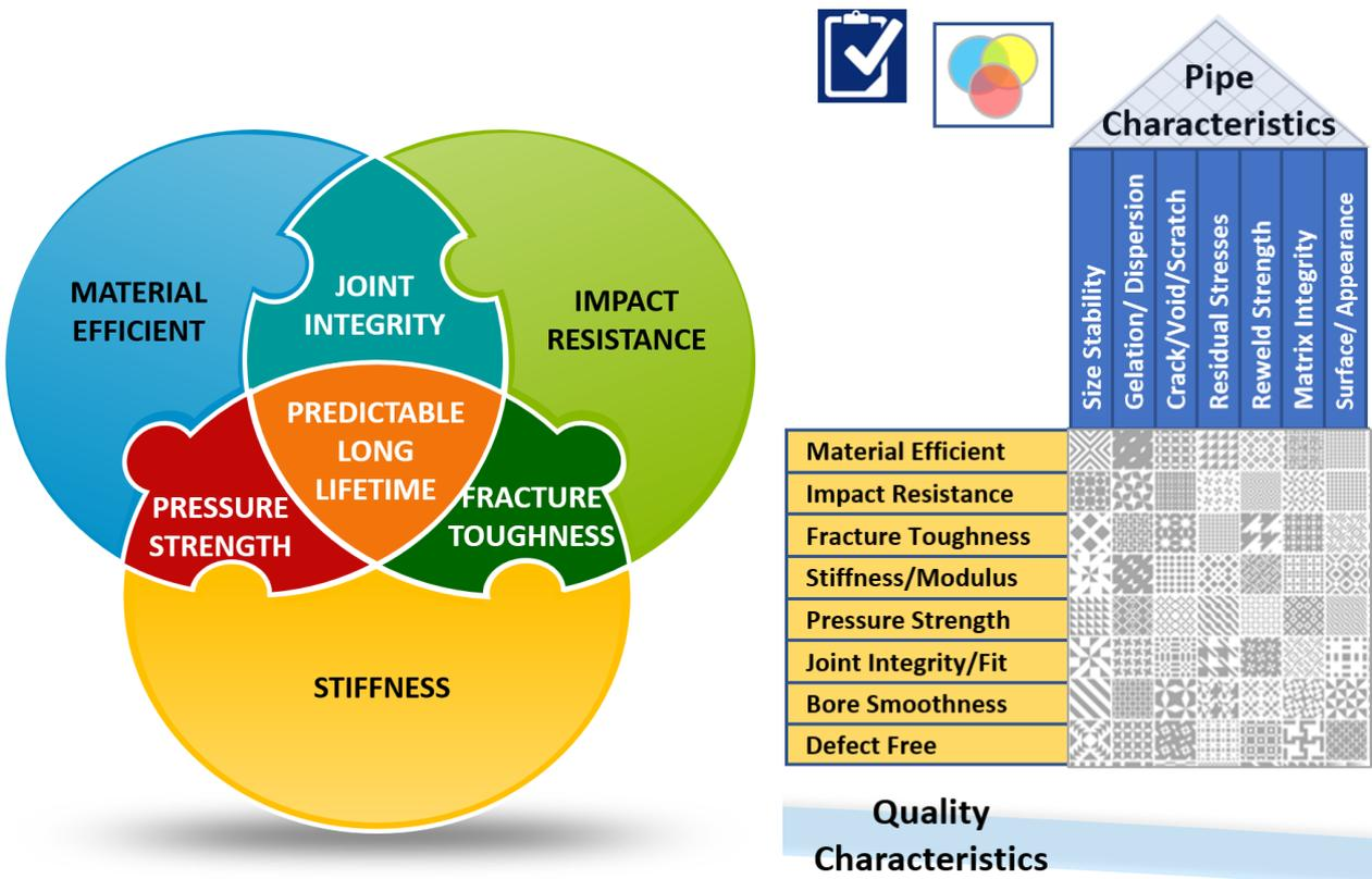
Impact Resistance and Stiffness combine to form Fracture Toughness. A Material efficient pipe with high Impact Resistance needs Joint Integrity. A pipeline that is Material Efficient still needs Pressure Strength through orientation or Stiffness through structure.
