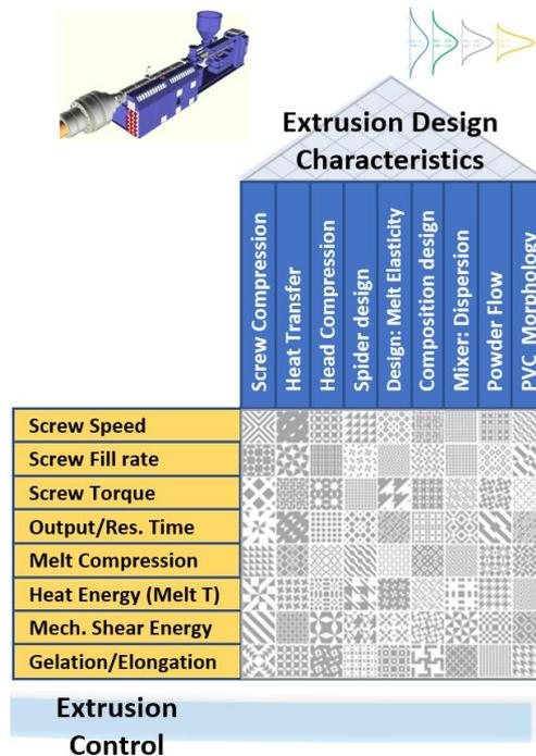
The Screw Speed and the Fill of the screw determine the Output.
