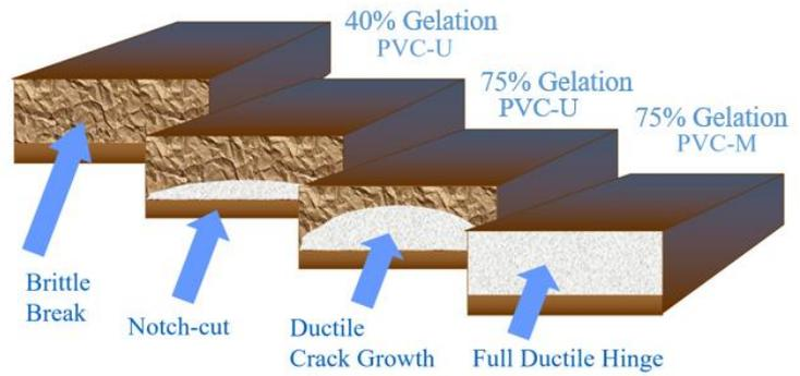
Figure 6: Fracture Toughness (crack resistance) measurement
