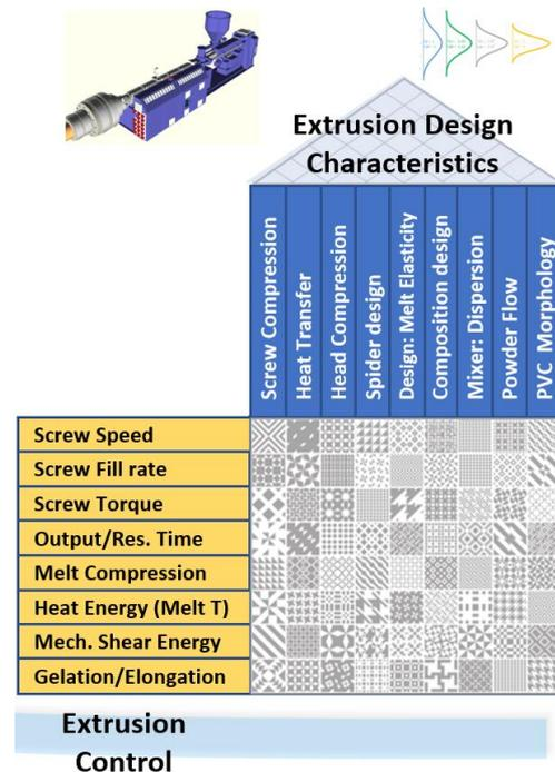
The Screw Compression design and the Barrel & Screws Heat Transfer determines the Material Dispersion. The Heat Transfer and the Head Compression design determine the Melt Elasticity for good reweld. The Head Compression and Screw Compression design is related to the PVC Morphology and Elasticity. Uniform Melt Flow with low variation for consistent uniform properties with no burning is the product of Material Dispersion, Melt Elasticity and PVC Morphology.
