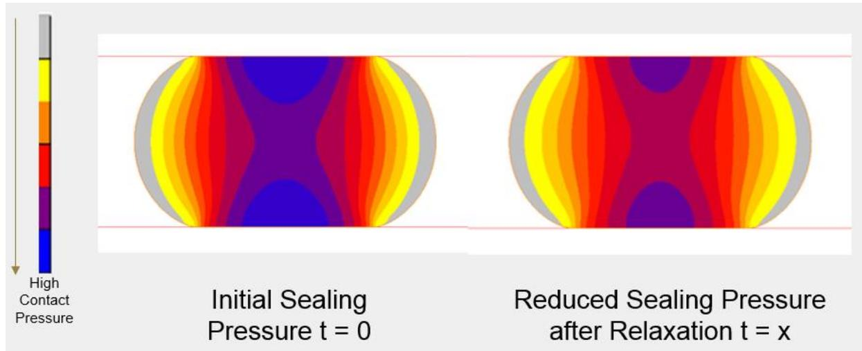
The illustration above shows the initial sealing pressure, achieved when the joint is first assembled, and the reduced sealing pressure after stress relaxation.
