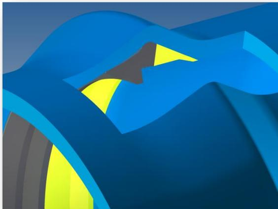
Integrated ‘Rieber’ System Joint
