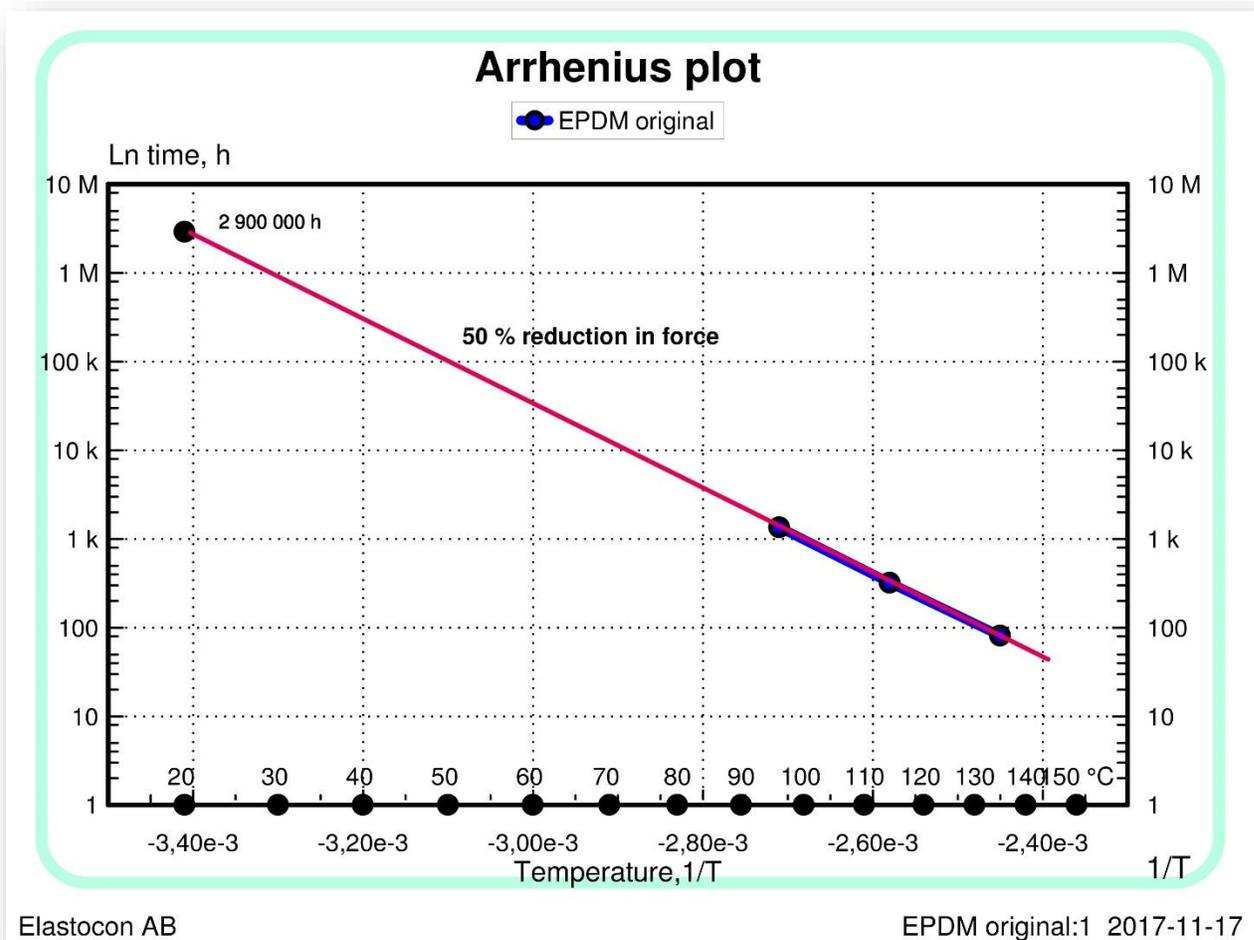
The threshold value is chosen as the maximum relaxation acceptable for the application. Commonly, 50% of the initial value is chosen (ref ISO 11346, section 6), but 30% and 40% were also measured.
