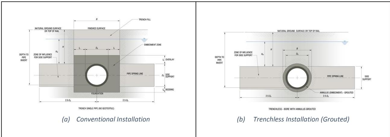
Figure 4 - Typical Conventional (Trenched) and Trenchless Installations
