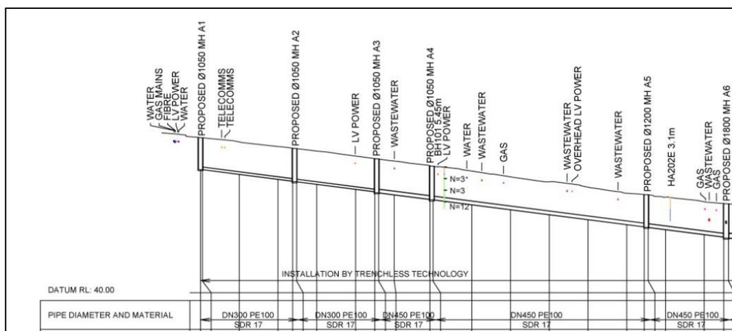
Figure 1 - Example Pipeline Design Longitudinal Section
