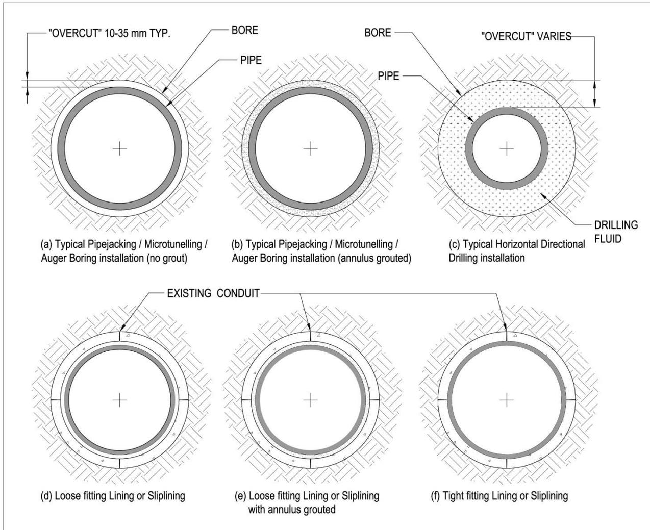
Figure 2 - Typical "pipe" installations using different trenchless installation methods
