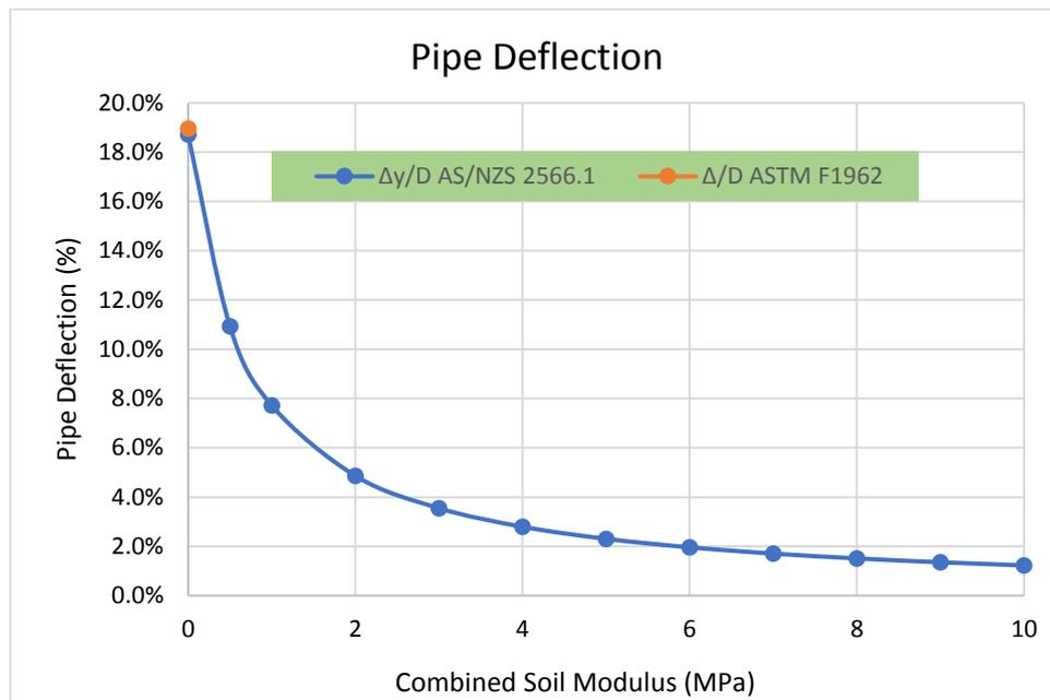
Figure 6 - Deflection of DN450 PE100 SDR17 Pipe for Different  $E'$  Values
