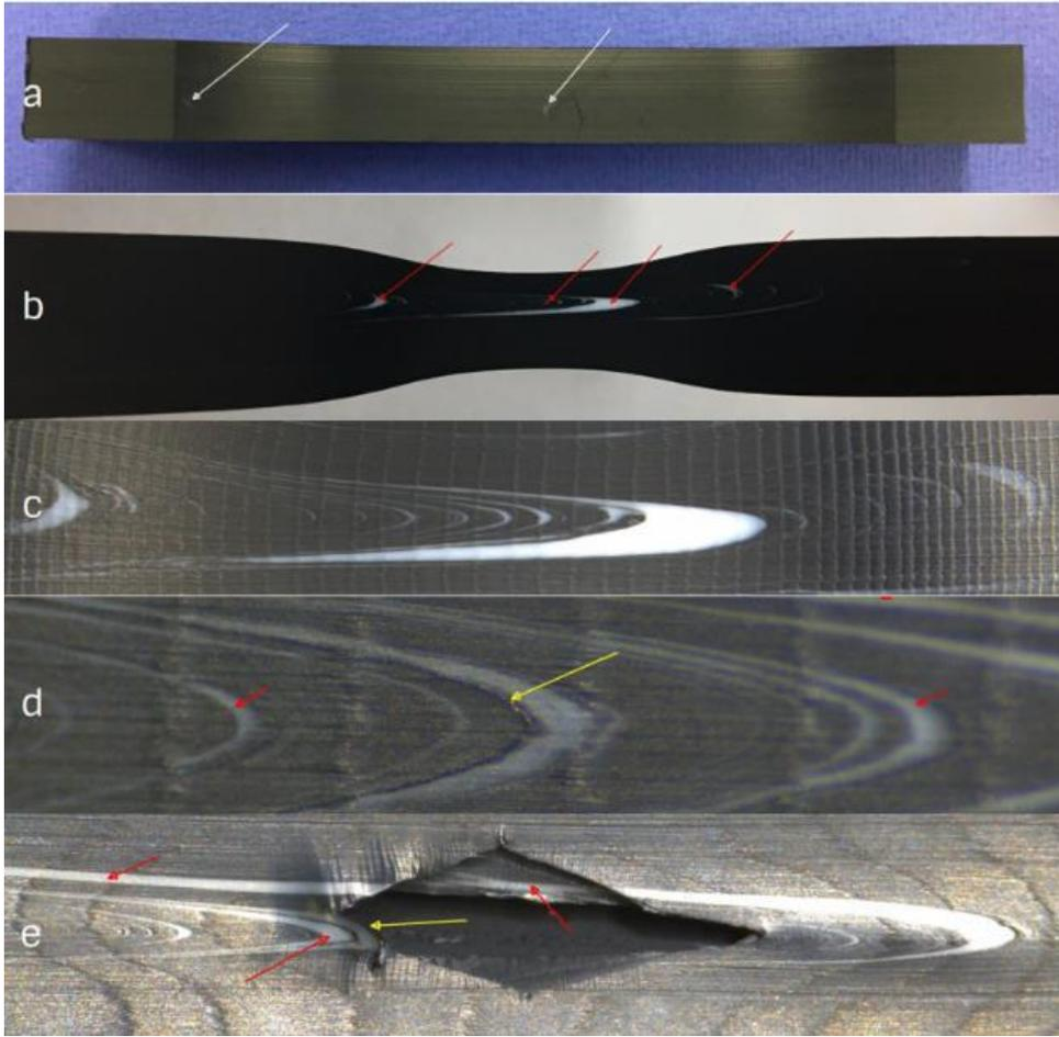
**Figure 3:** Propagation of windows to fracture: (a) tensile specimen before testing—white arrows indicate ‘windows’ visible to the naked eye; (b) tensile specimen after yield (20% elongated)—red arrows show windows curled towards the tensile direction; (c) tensile specimen (40% elongated); (d) interface separation at the edge of windows marked with a yellow arrow; (e) fracture occurrence at the interface separation (yellow arrow).
