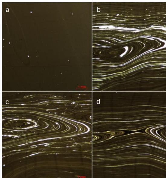
Figure 1: Microscopy images of 15  $\mu\text{m}$  slices (cross-flow) taken from pipe specimens: (a) Sample 1, (b) Sample 2, (c) Sample 3 and (d) Sample 4
