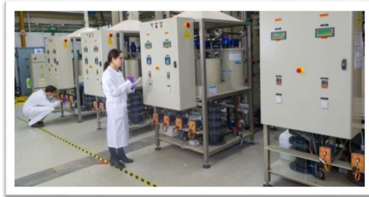
**Figure 4.** Accelerated ageing installation used for small scale screening test and pipe performance long-term test.
